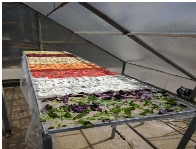
Figure 7. View of a solar dryer greenhouse device in drying mode
